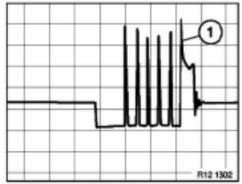
The ignition timing will be progressively advanced assisting the engine in coming up to speed. As the engine speed approaches idle rpm, the timing remains slightly advanced to boost torque. When the engine is at idle speed, minimum timing advance is required. This will allow faster engine and catalyst warm up. The multiple pulsing switches to single pulse when engine speed >1350 RPM (varied with engine temperature).
